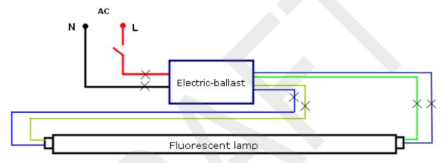
Step3. Install LED tube into lighting fixture with below one (Type I) wiring method refer to the label on the tube.
